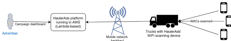
Figure 2: HaulerAds scanners detect mobile devices near the OOH advertisement and send data through the mobile backhaul to the HaulerAds platform
