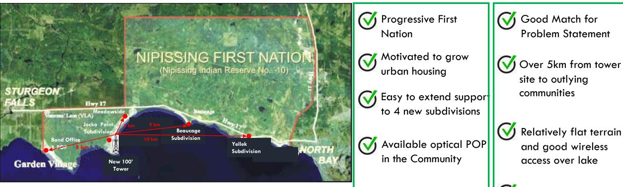
Single tower design made possible by hybrid TVWS and 5GHz radio design for flat terrain, broadcast across lake, and clear access to distributed lakeshore community.
